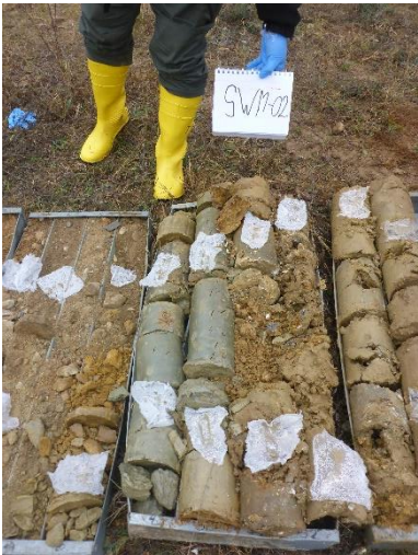
Photo 4: Groundwater monitoring well 2 - drilled materials
