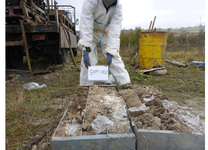
Photo 3: Groundwater monitoring well 1 - drilled materials
