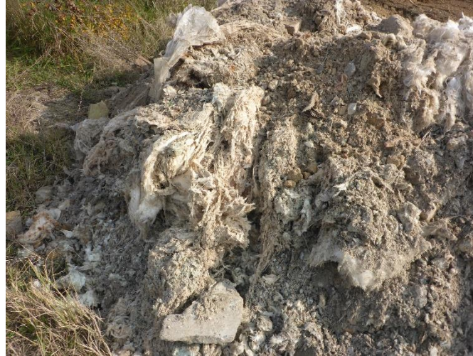
Photo 2: Excavated materials consisting of glass wool and concrete
