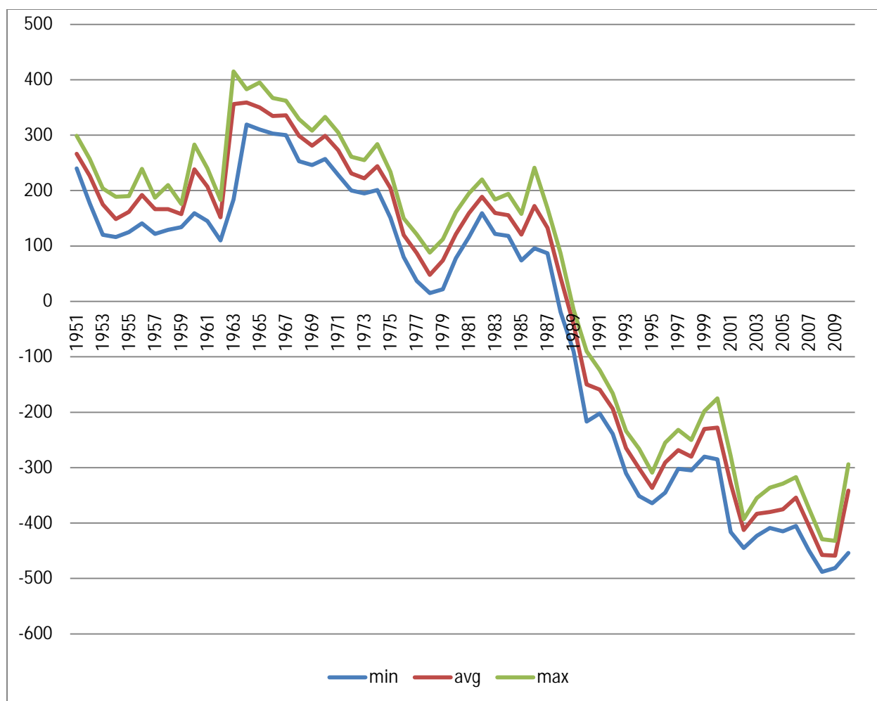
Oscillation of the lake water level at Macro Prespa - station Stenje "0" 847.48 m a.s.l. for the time period 1951-2010 (source: National Hydrometeorological Services – Skopje)
