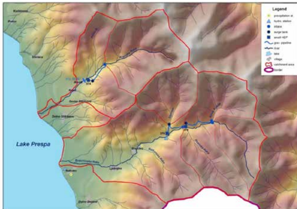
Figure ???? Small HEP in river Brajcinska (No. 375, 376) and river Kranska (No. 374). Source: Development of Prespa Lake Watershed Management Plan (UNDP, 2012)
