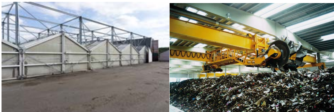
Figure 21 Examples for in-vessel composting
