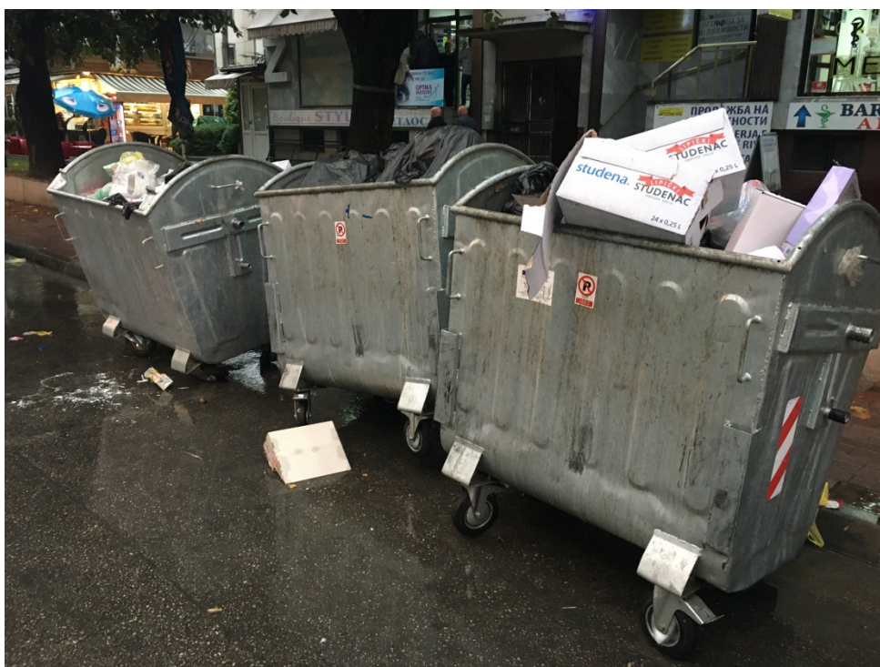
Figure 7 Steel containers 1.1 m 3 used in the project region without lids and partly broken swivel caster wheels
