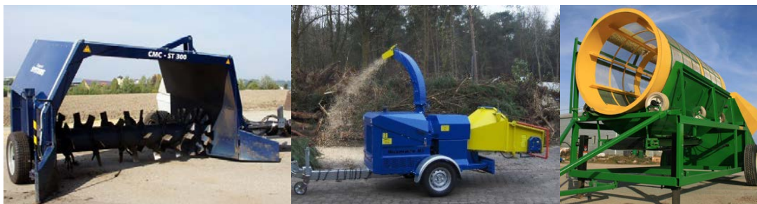
Figure 20 Pull-type windrow compost turner 8 (l.), chipper 9 (middle), drum screen 10 (r.)
