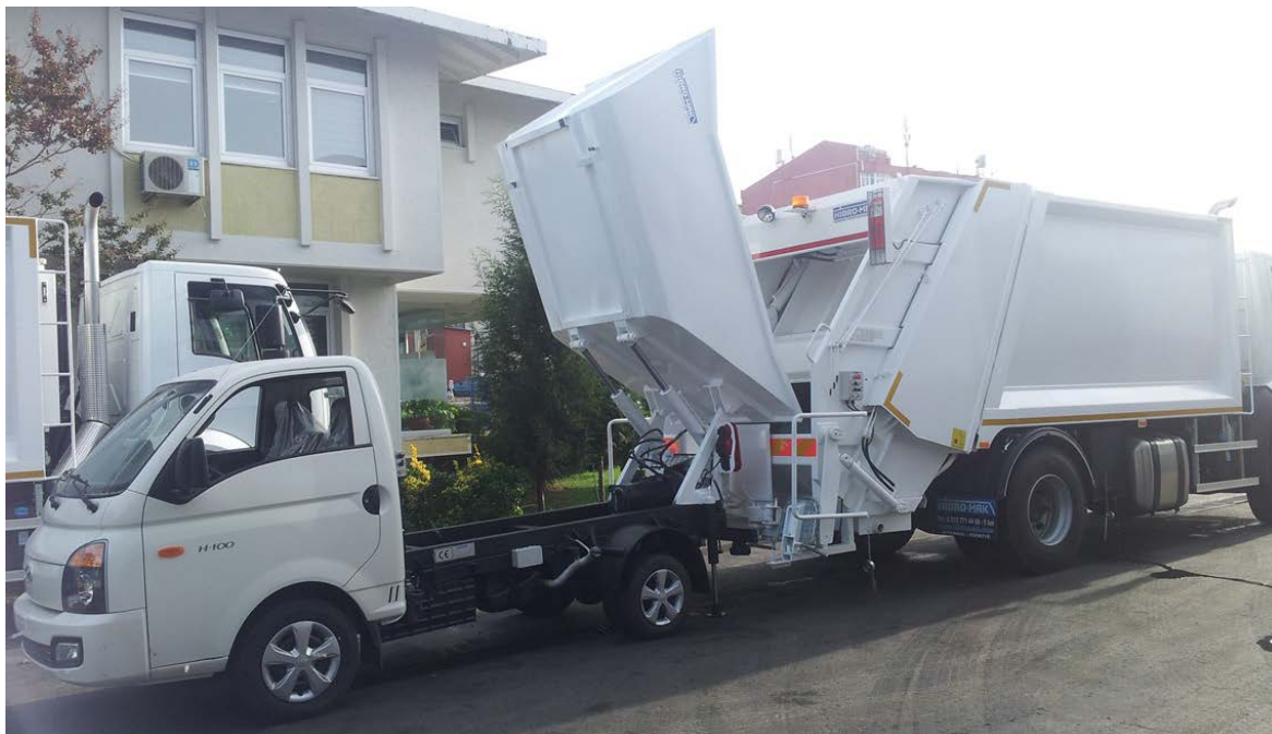
Figure 11 Secondary collection: A small waste truck off-loads the waste into a larger compaction truck
