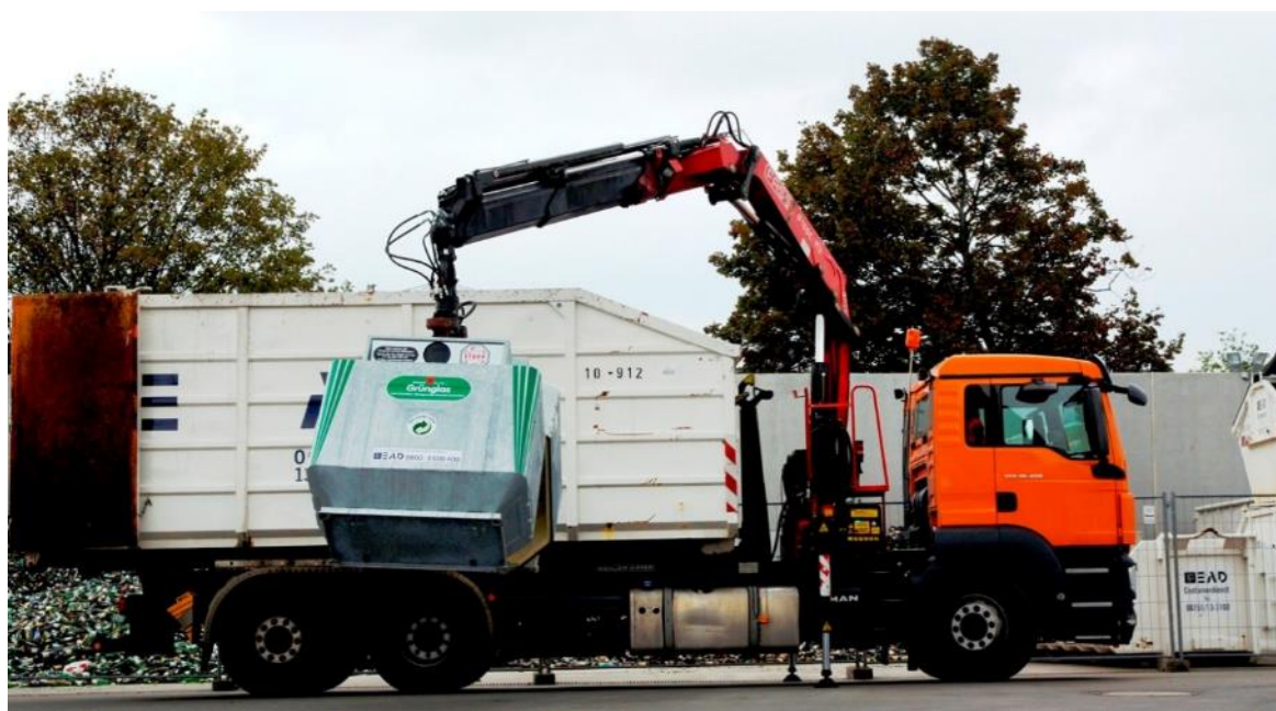
Figure 26 Emptying of a depot container with hoist hook
