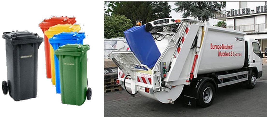
Figure 10 Small waste containers and collection vehicle with suitable lifting device
