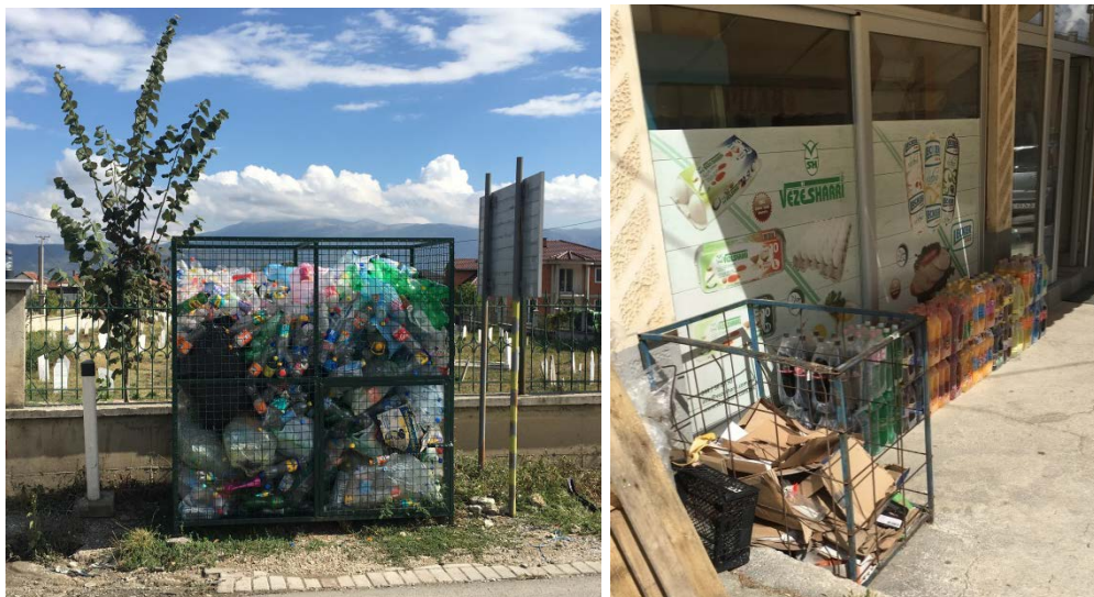
Figure 13 Mesh wire boxes for separate collection of PET bottles and cardboard waste
