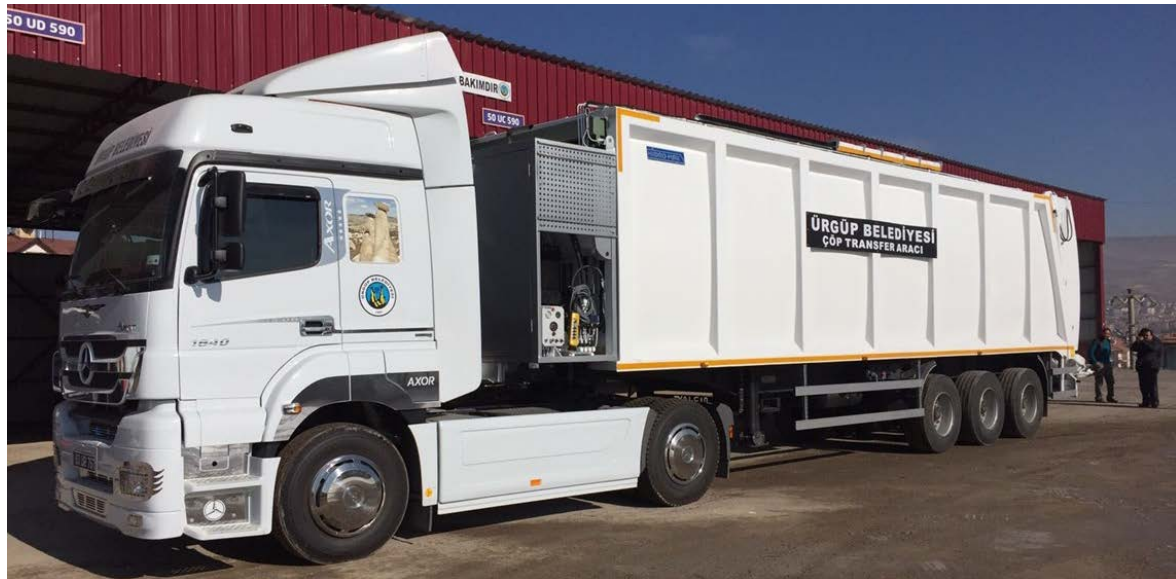
Figure 16 Tractor and a semi-trailer with a self-driven compaction unit
